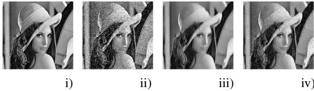
Fig. 2. i) Original Image. ii) Noisy image. iii) Reconstructed image ( K = 6 ). iv) Reconstructed image ( K = 10 ).
